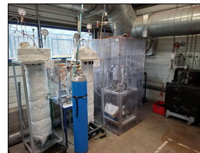
HP- Immersion tests in large-volume autoclaves
