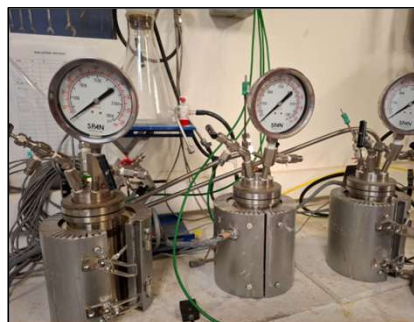
HP- Immersion tests in small autoclaves
