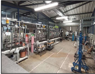
Test room for tensile test (constant load, SSRT, Ripple load....)
