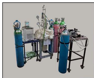
Batch autoclave for pre-soaking at HP/HT
