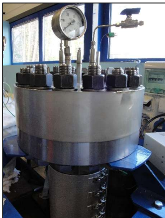
Batch autoclave for pre-soaking at HP/HT
