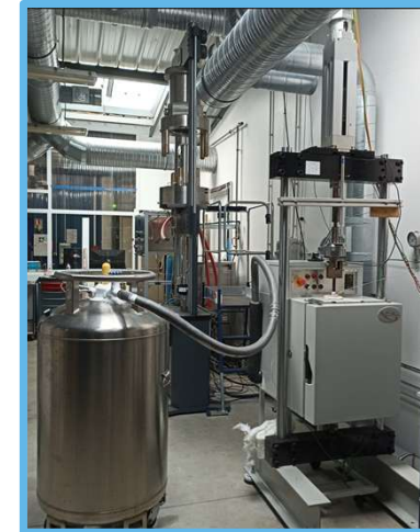
SSRT at cryo-Temperatures
