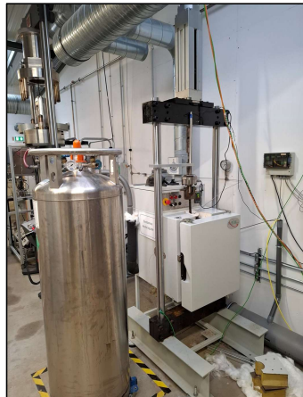
SSRT at high/ low temperatures
